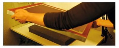
The styropor has to be in a size that will fit the inner frame and must be so thick that the screen lays directly and strong to it!
