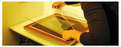
Place a clear glass over the foil, it must be big as the screen and it must press the foil completely to the screen. Now you can place the UV lamp over the screen. Approx for our screen size in a distance of 65cm.
